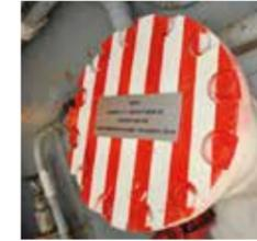
**1** Removal of the blind flange gives access to the sounding or vent pipe.
