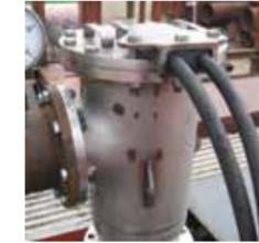
**2** The T-piece with discharge hose connection is connected to the flange.
